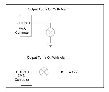
Please note that the outputs are reverse logic: the output will supply current when there is NO error.
