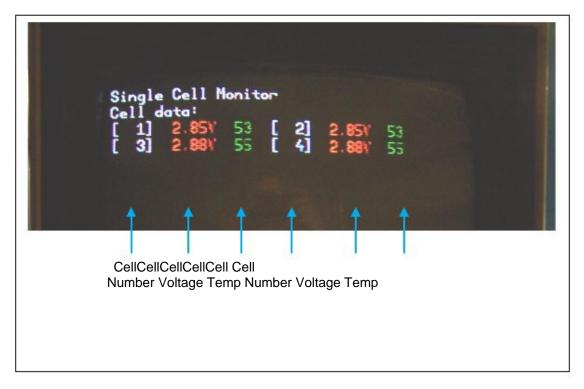
The data for up to 20 cells is displayed on each page as two columns of up to 10.
